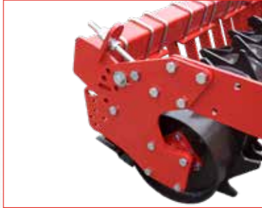
RULLO PACKER (Ø 406-464-500-550) PACKER ROLLER • ROULEAU PACKER • PACKERWALZE • RODILLO PACKER
